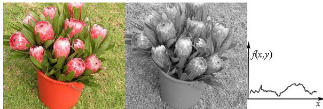
Figure: Variations of grey values for different x -positions along a line y = \text{const}
